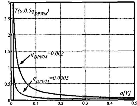
Fig. 11. Magnitude loop gain  $T(a, \epsilon_{DPWM})$  at  $f_s$  for two DPWM quantization levels  $q_{DPWM}$  in the example of Section VI.B.
