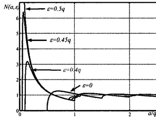
Fig. 6. Describing function of a quantizer for several different values of the offset  $\varepsilon$ .
