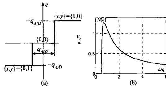
Fig. 13. Characteristic (a) and the describing function (b) of the A/D converter in Fig. 12.
