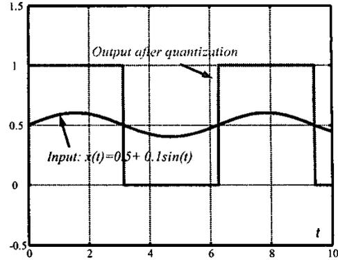
Fig. 5. Small amplitude sinusoidal signal becomes square wave signal with much bigger amplitude when the DC offset  $\varepsilon$  of the input sinusoidal signal matches the transition point ( $0.5q$ ) between two quantization bins.
