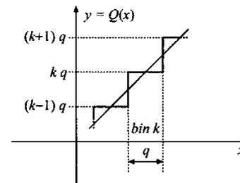
Fig. 2. Quantizer characteristic.
