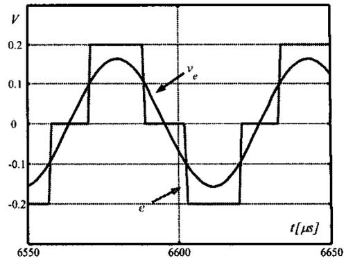
Fig. 9. Steady-state waveforms  $v_e$  at the A/D input and  $e$  at the A/D output in the example of Section VI.A.
