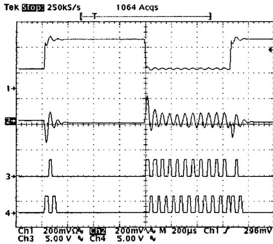
Fig. 14. Experimental waveforms in the example of Section VI.C; Ch1: load current  $i_{oad}$  [200mA/div], Ch2: ac-coupled output voltage  $v_{oad}$ , Ch3: A/D comparator output  $y$ , Ch4: A/D comparator output  $x$ .
