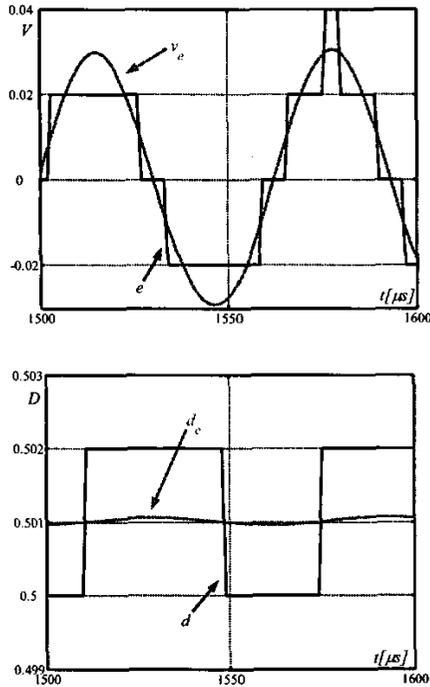
Fig. 10. Top: waveforms  $v_e$  and  $e$  before and after A/D quantization. Bottom: duty-cycle command  $d_c$  at the DPWM input, and the quantized duty-cycle command  $d$  in the example of Section VI.B.
