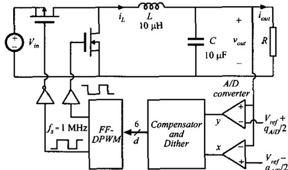
Fig. 12. Experimental digitally-controlled 1 MHz buck converter [11].
