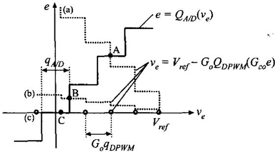
Fig. 3. Graphical solution of the static model for the digitally controlled converter of Fig. 1, for three DC compensator gains  $G_{co}$ : (a) small  $G_{co}$ , (b) large  $G_{co}$ , and (c)  $G_{co} \rightarrow \infty$ .
