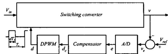
Fig. 1. Digitally controlled DC-DC switching power converter.
