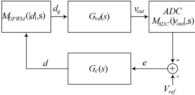
Fig. 2. Linear model of SMPS feedback loop
