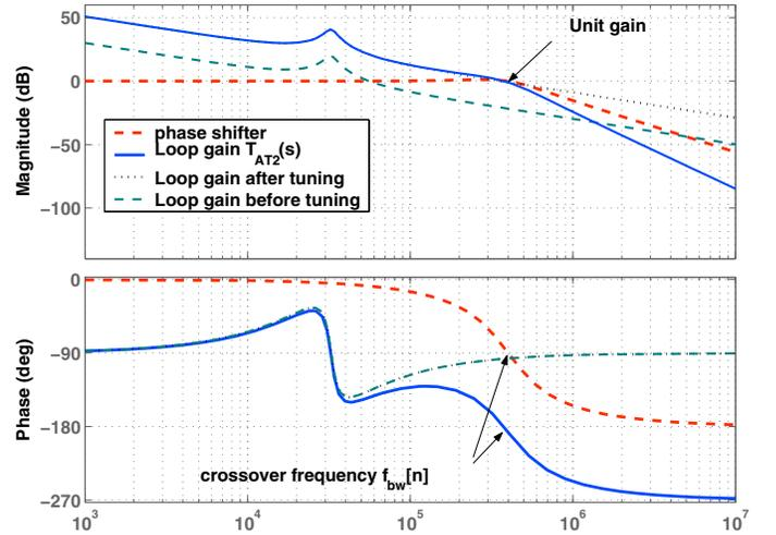
Fig. 5. Bode plots of systems during second step tuning
