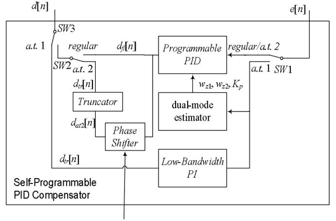
Fig. 3. Self-programmable PID compensator block diagram
