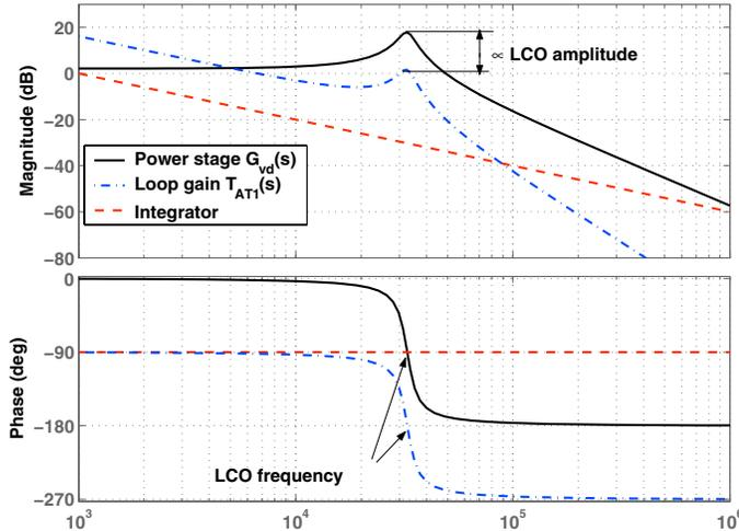
Fig. 4. Bode plots of systems during first step tuning
