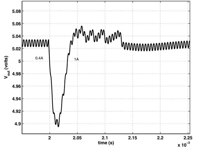
Fig. 7. Transient response of the auto-tuned system to a load current change from 0.4A to 1A
