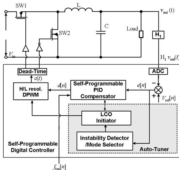
Fig. 1. Self-programmable SMPS system block diagram
