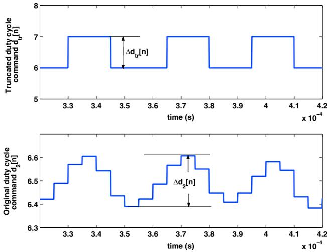
Fig. 6. Input (bottom) and output (top) of the nonlinear element (DPWM quantizer)
