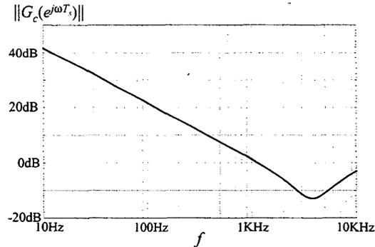
Fig. 9. Magnitude response of the digital PID regulator.
