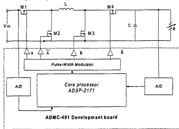
Fig. 1. Non-inverting buck-boost converter with a digital controller.
