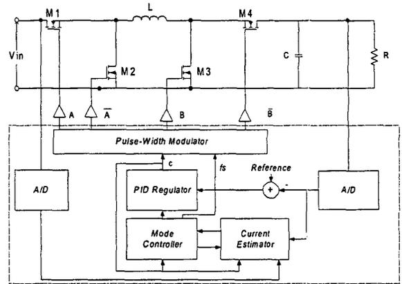
Fig.3. Controller configuration.
