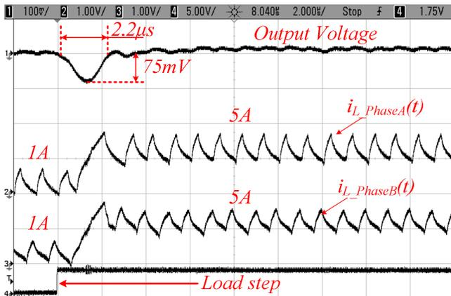
Fig.5. Transient response on a two-phase interleaved buck converter for an 8A light-to-heavy load step change. Ch.1: Output voltage (100 mV/div); Ch2 and 3: Signals from current sense circuit; Ch.4: Load step command. The time scale is 2µ/div.
