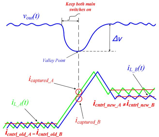
Fig. 4. The key waveforms of a two-phase interleaved buck converter during a light-to-heavy load transient. Top: output voltage of the converter; Bottom: inductor phase currents.
