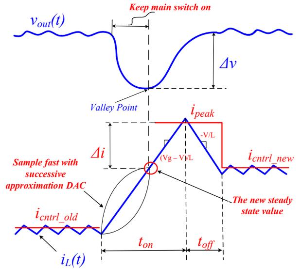
Fig. 3. The key waveforms of a single-phase power stage during a light-to-heavy load transient. Top: output voltage; Bottom: the inductor current.
