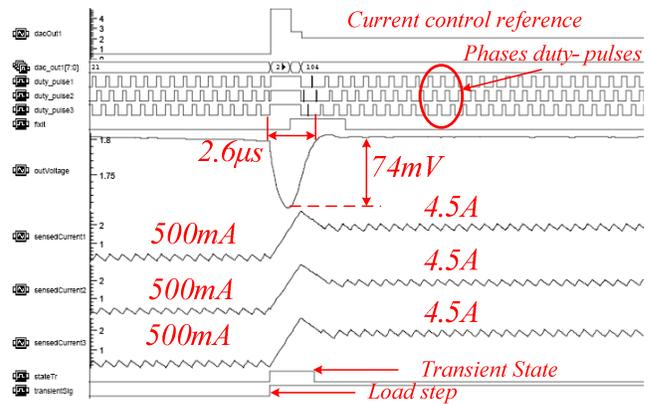
Fig. 10. Load transient response of a 3-phase interleaved system (simulation results).
