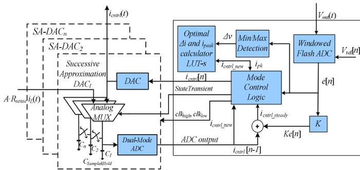
Fig. 2. Block diagram of the voltage loop
