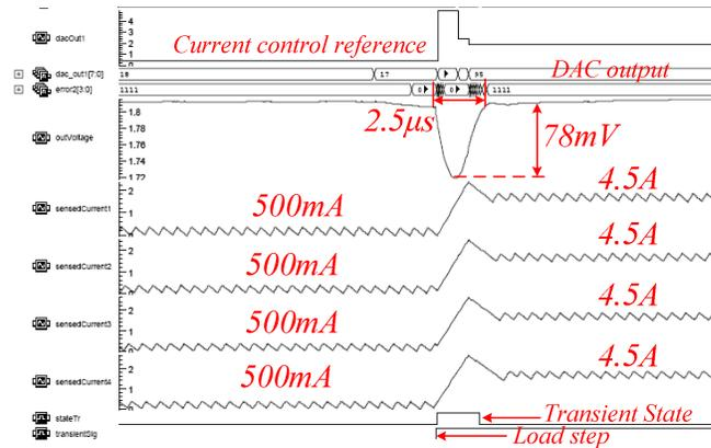
Fig. 11. Load transient response of a 3-phase interleaved system (simulation results).
