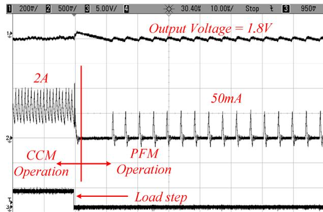
Fig.9. Transition between CPM and PFM modes for a heavy-to-light load transient. Ch.1: Output voltage (200mV/div); Ch.2: Signal from current sense circuit of a phase; Ch.3: Load step signal. The time scale is 10µs/div.
