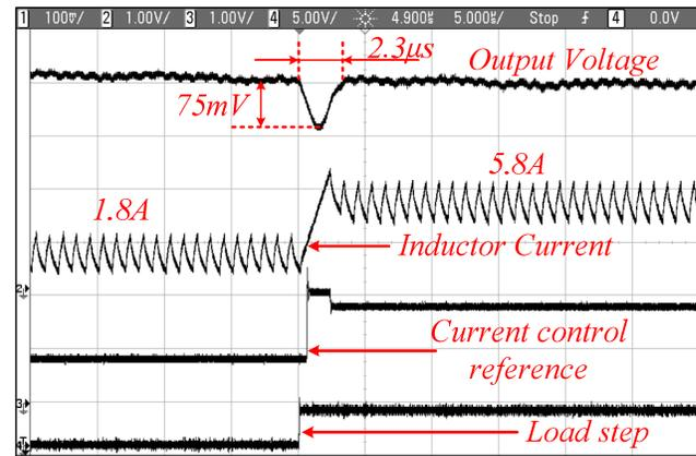
Fig.6. Key controller and power stage waveforms during a light-to-heavy load transient. Top: Output voltage (100 mV/div); Ch.2: Signal from a current sense circuit; Ch.3: Current control reference  $i_{ref}(t)$ ; Ch.4: Load step command. The time scale is 5µ/div.
