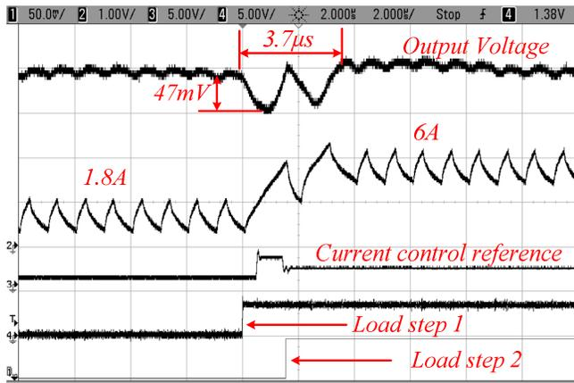
Fig. 8. Two consecutive transients using CT-DC. Top to bottom: Output voltage (50mV/div); Sensed inductor current; Current control reference; First load change command ; Second load change command. The time scale is 2µs/div.
