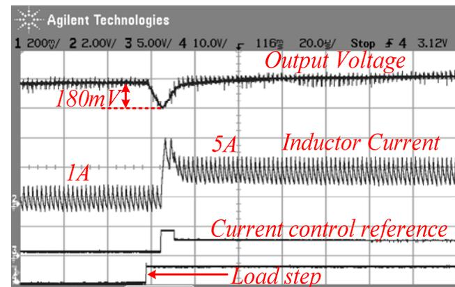
Fig. 7. Operation of current protection. The waveforms from top to bottom are: Output voltage (200mV/div); Amplified inductor current; Current control reference; Load step signal. The time scale is 20µ/div.
