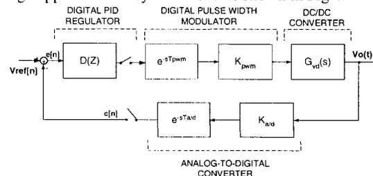
Fig.4. Block diagram of the digital control system
