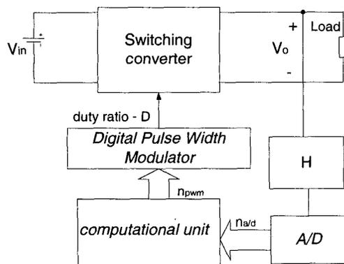
Fig.1. Digital control system for a switching converter
