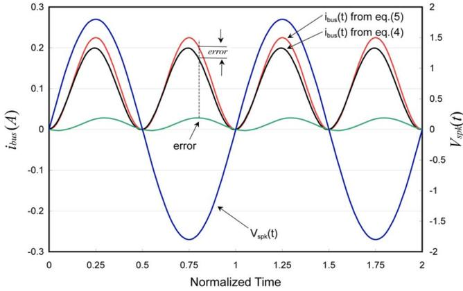
Fig. 10. Illustration of the error in the bus current estimation arising from the approximation  $Y(j\omega) \approx 1/R$ .
