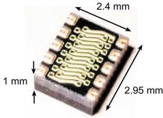
Fig. 19. Custom chip-size-module (CSM) package that includes the micro inductor from Fuji Electric Advanced Technology Company, Ltd.
