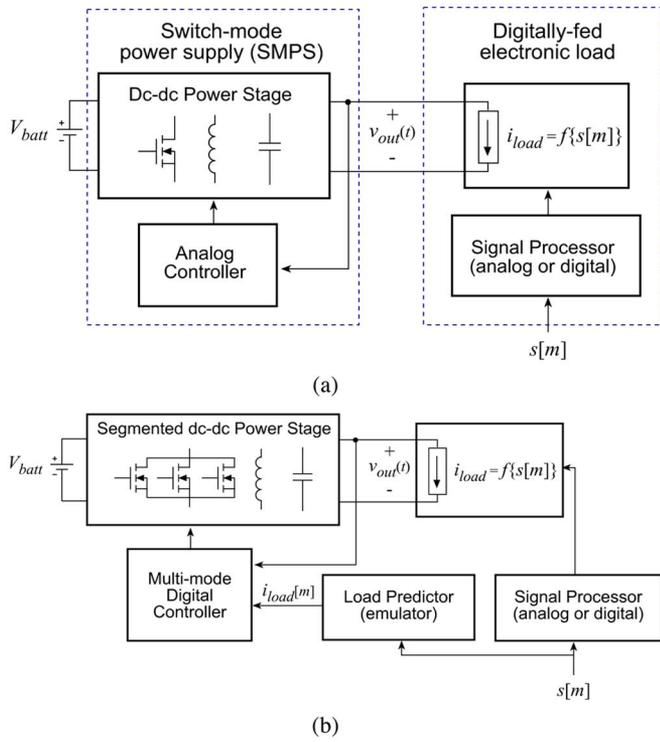
Fig. 1. (a) Conventional power system for supplying digitally fed electronic loads. (b) Digitally controlled predictive efficiency optimization system.
