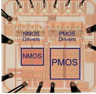
Fig. 18. Chip micrograph for the segmented power-stage IC.
