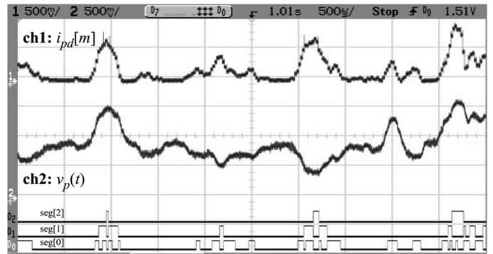
Fig. 13. Predicted dc–dc load current, speaker terminal voltage, and segment enable codes during audio playback. A segment-code of  $seg = 0$  indicates that the converter operates in PFM mode. Ch-1:  $i_{pd}[n]$ , 500 mV/div; Ch-2:  $v_p(t)$ , 500 mV/div.
