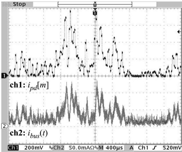
Fig. 11. Predicted and actual dc–dc converter load current with a speaker load. The predicted current  $i_{pd}[m]$  is shown using an 8-b flash D/A. Ch-1:  $i_{pd}[m]$ , 200 mV/div; Ch-2:  $i_{bus}(t)$ , 50 mA/div.
