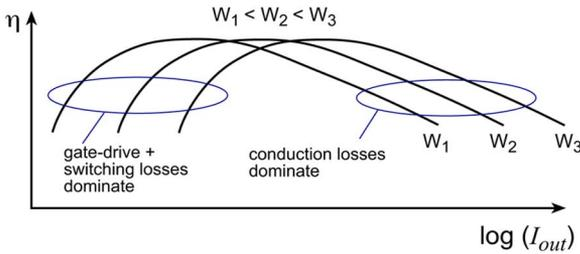
Fig. 8. Efficiency curves for increasing power-stage transistor size.
