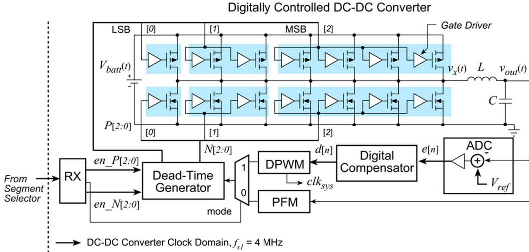
Fig. 7. Digitally controlled dc–dc controller architecture.
