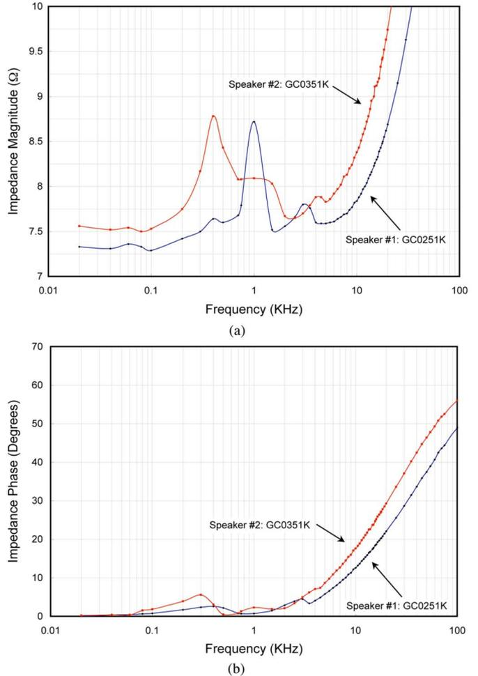
Fig. 9. Measured (a) magnitude and (b) phase of the speaker impedance.
