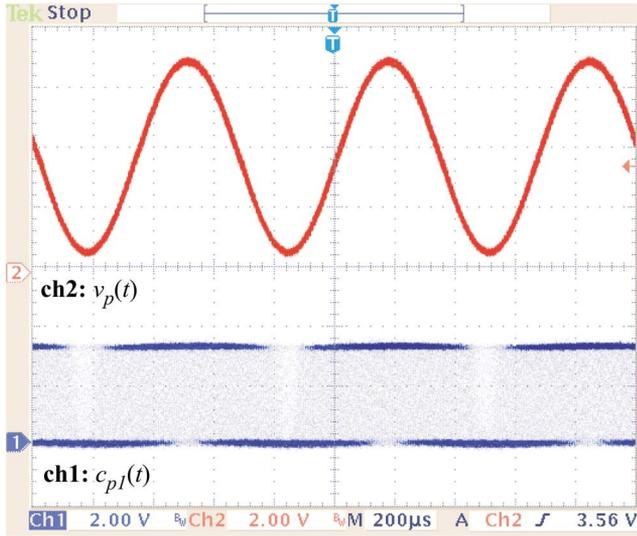
Fig. 3. Output of the class-D amplifier for a 1.5-kHz single tone audio input. Ch-1:  $c_{p1}(t)$ , 2V/div; Ch-2:  $v_p(t)$ , 2V/div.
