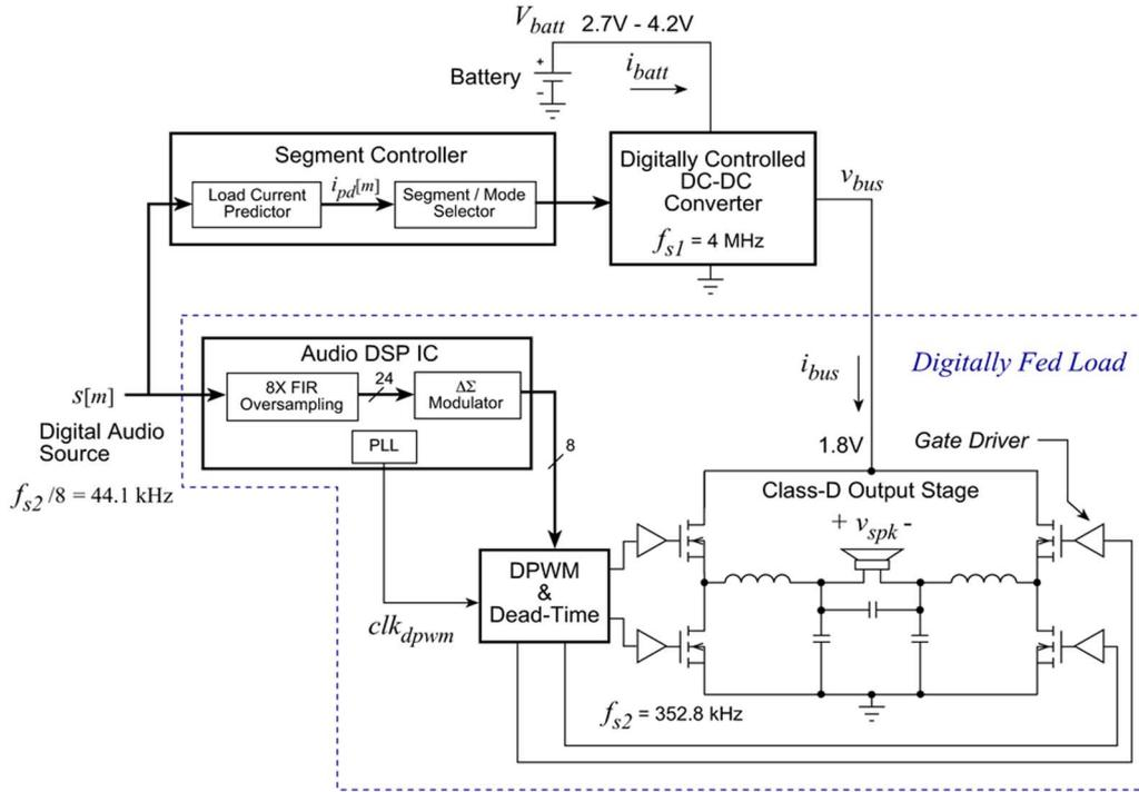
Fig. 4. Simplified diagram of the dc-dc powered class-D audio amplifier system. A sensorless digital current predictor is used to dynamically optimize the power-stage sizing and switch between PFM/PWM based on the digital audio stream.
