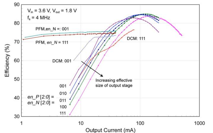
Fig. 17. Measured efficiency versus load with different segment enable codes and modes of operation for the power-stage IC.
