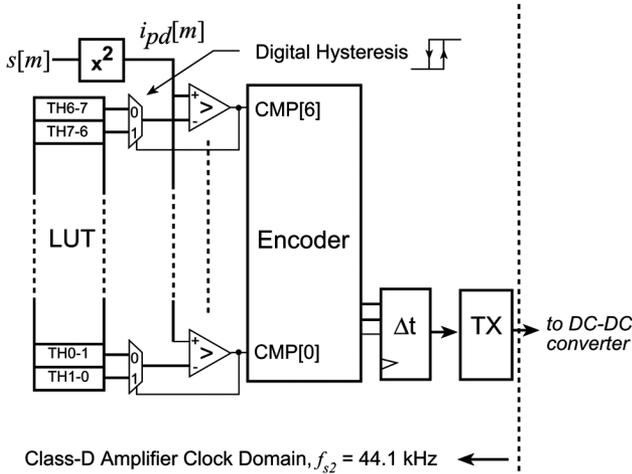
Fig. 6. Segment controller and digitally controlled dc–dc converter communicate using an asynchronous interface.
