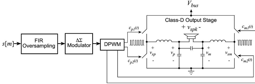
Fig. 2. Simplified architecture of a digital class-D amplifier with an H-bridge power-stage.
