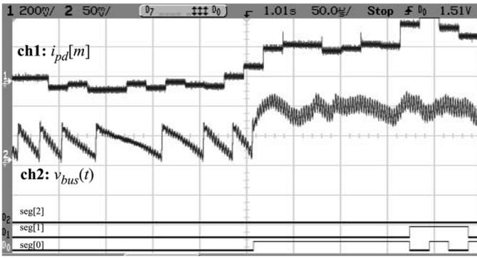
Fig. 15. Predicted dc-dc load-current and regulated output voltage during a transition from PFM to PWM mode. Ch-1:  $i_{pd}[n]$ , 200 mV/div; Ch-2 (ac-coupled):  $v_{bus}(t)$ , 50 mV/div.
