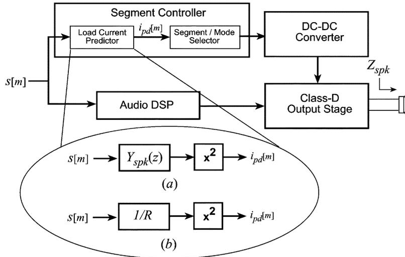
Fig. 5. Load prediction implementation when the speaker is modeled as (a) a general admittance  $Y_{spk}(z)$  and (b) a resistor.
