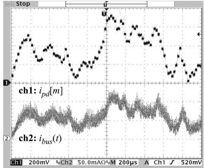
Fig. 12. Predicted and actual dc–dc converter load current with a speaker load. Ch-1:  $i_{pd}[m]$ , 200 mV/div; Ch-2:  $i_{bus}(t)$ , 50 mA/div.
