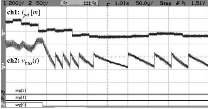
Fig. 14. Predicted dc-dc load-current and regulated output voltage during a transition from PWM to PFM mode. The load-current varies continuously during audio playback; hence, this does not correspond to a traditional load step response. Ch-1:  $i_{pd}[n]$ , 200 mV/div; Ch-2 (ac-coupled):  $v_{bus}(t)$ , 50 mV/div.
