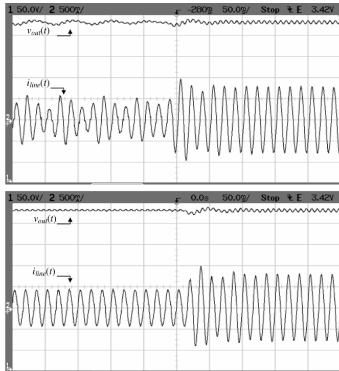
Fig. 16. Output voltage and input current during a 30–60 W load transient in the experimental PFC with the fixed dead-zone controller (top), and the self-adjustable dead-zone controller (bottom). The time scale is 100 ms/div, Ch1: v_{out}(t) , 50 V/div, Ch-2: i_{line}(t) , 0.5 A/div.
