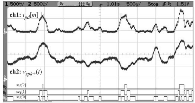
Fig. 10. Predicted DC-DC load current: (ch1) speaker terminal voltage (ch2); and segment enable codes during audio playback. A segment code of  $seg=0$  indicates that the converter operates in PFM mode
