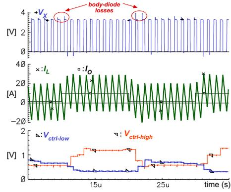
Fig. 5. Transient waveforms of ZVS-QSW buck converter with DTLLs under a dynamic load (1.5A-10A).
