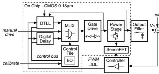
Fig. 7. Block diagram of the ZVS-QSW buck converter with integrated DTLLs.
