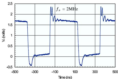
Fig. 9. Measured voltage waveform at node X of the ZVS-QSW converter. Body-diode losses occur due to the shorter than ideal dead-time.
