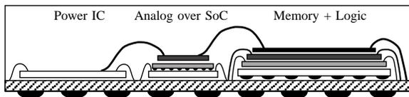
Fig. 1. Representation of Multi Dimensional Die-Integration System Chip [1].
