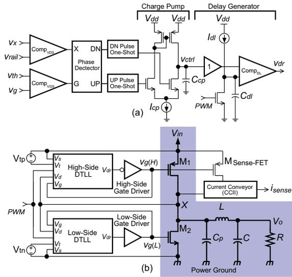
Fig. 3. (a) ZVS-QSW buck converter with Dead-Time-Locked-Loops. (b) Circuits inside one of the DTLL blocks.
