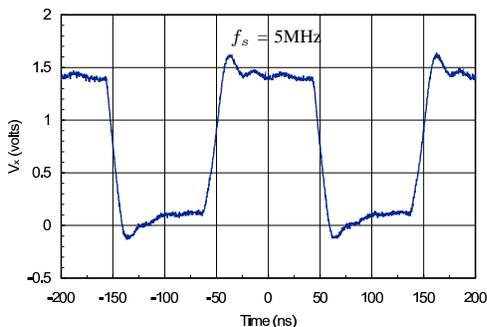
Fig. 10. Measured voltage waveform at node X of the ZVS-QSW converter. Proper gate-drive timing eliminates body-diode conduction after resonant transitions.
