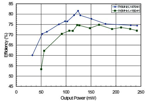
Fig. 11. Measured efficiency of the ZVS-QSW converter for  $V_{in}=2V$ ,  $V_o=1.4V$ .
