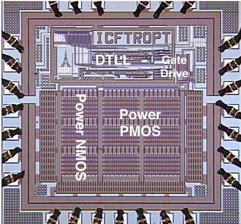
Fig. 8. A micrograph of the 0.18µm CMOS 1.56mm<sup>2</sup> integrated ZVS-QSW DC-DC converter chip.
