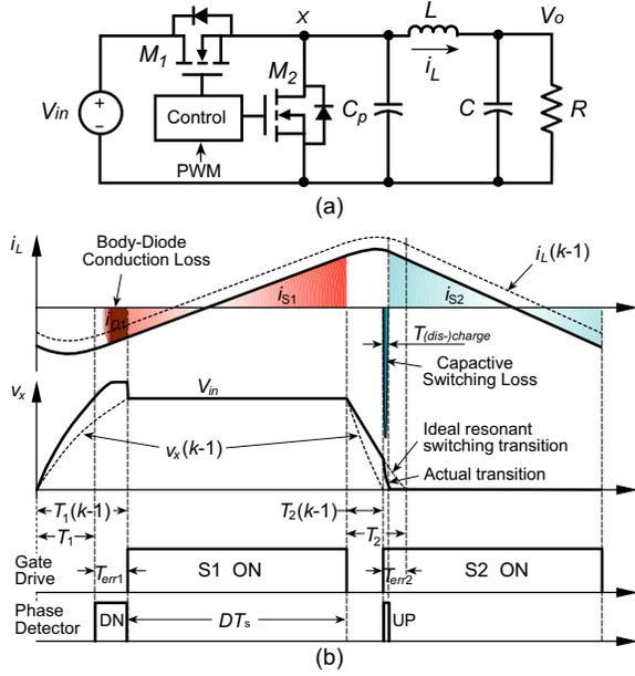
Fig. 2. (a) ZVS-QSW buck converter. (b) Load transient leads to dead-time errors and switching loss. The period  $k-1$  has ideal dead-times.
