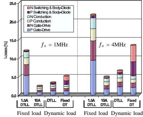
Fig. 6. On-Chip losses with DTLL/fixed dead time.  $V_o=1.3V$ , devices optimized @10A, for 1 and 4MHz.
