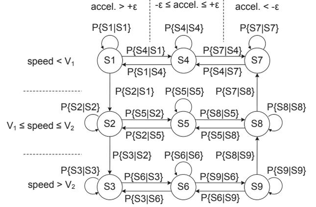
Fig. 4. The drive-cycle is represented as a Markov process with nine states.  $P\{S_n|S_m\}$  represents the probability of entering state  $n$  from state  $m$ .
