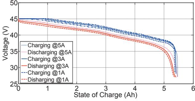
Fig. 5. Li-ion battery charge and discharge curves.
