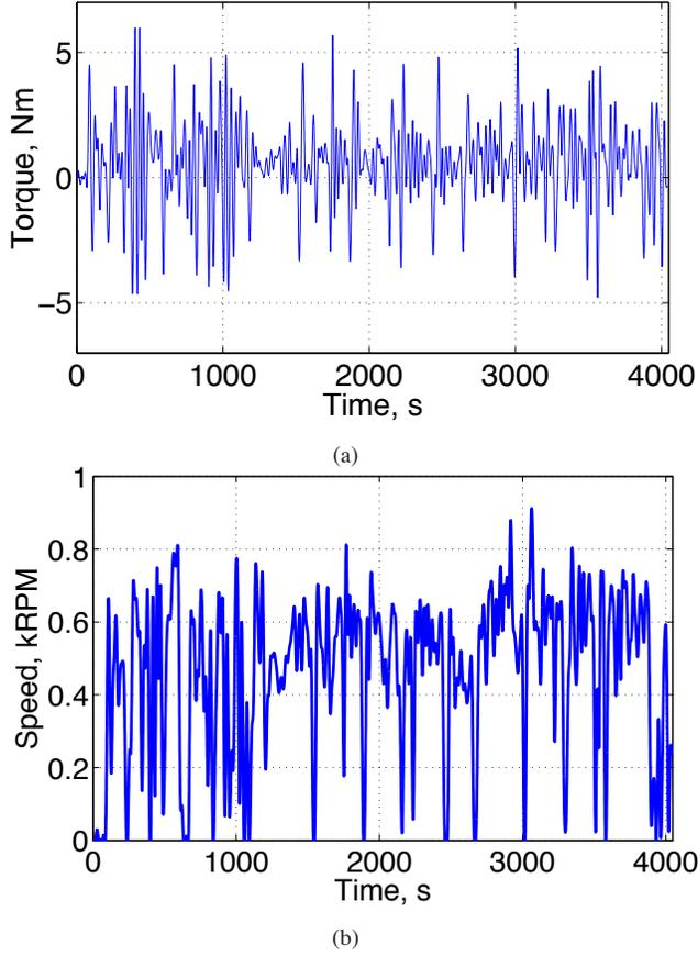
Fig. 2. Drive-cycle (a) torque and (b) motor speed data.
