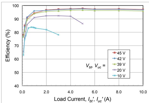
Fig. 9. Measured efficiency for the dc-dc converters with  $V_{bus} = 50.4$  V.
