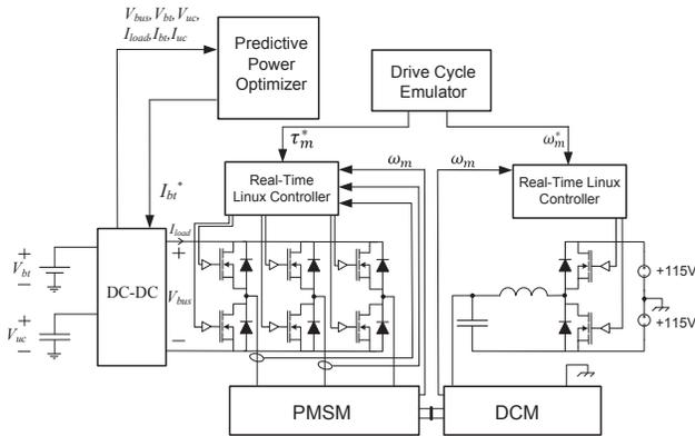
Fig. 8. Experimental system used to evaluate the PPO algorithm.
