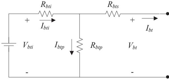
Fig. 6. Energy storage device model.
