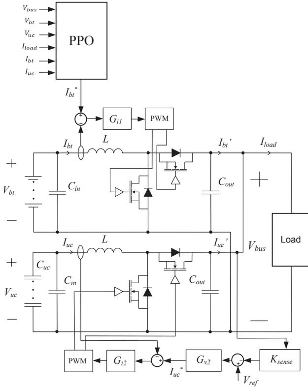
Fig. 1. Architecture for the hybrid u-cap/battery energy source.
