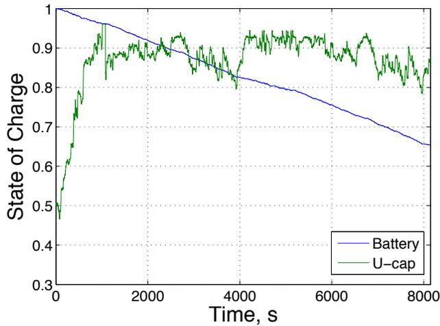
Fig. 10. Experimental battery and u-cap SOC.
