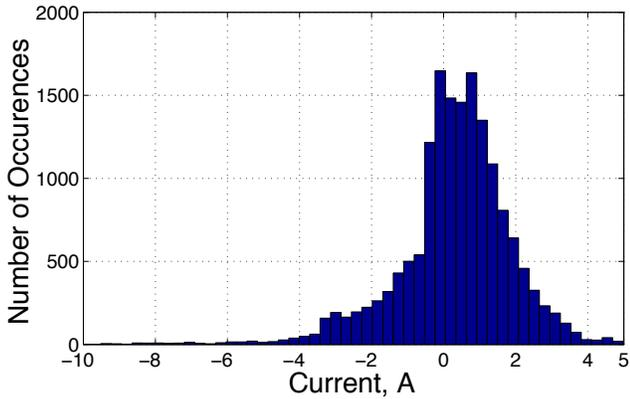
Fig. 3. Histogram of the load current for an LEV drive-cycle.
