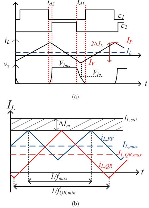
Fig. 2. (a) Ideal waveforms for ZVS operation. The optimal  $t_{d1}$  and  $t_{d2}$  depend on  $I_v$  and  $I_p$  respectively. (b) Inductor current constraints.
