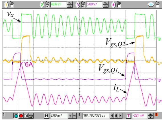
Fig. 7. Measured steady state waveforms of the converter operating in PFM mode. f-1:  $V_{gs,Q2}$ , 5 V/div; ch-2:  $v_x$ , 49.6 V/div; ch-3:  $V_{gs,Q1}$ , 5 V/div; f-4:  $i_L$ , 2 A/div.
