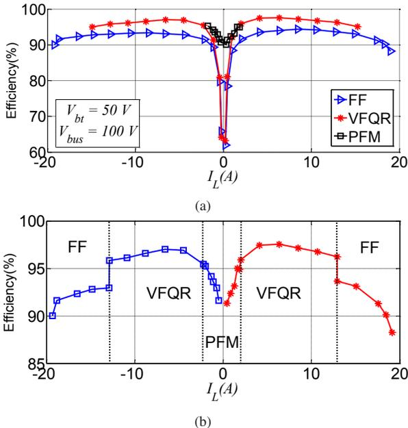
Fig. 8. Measured efficiency in (a) different modes of operation and with (b) Tri-mode converter.
