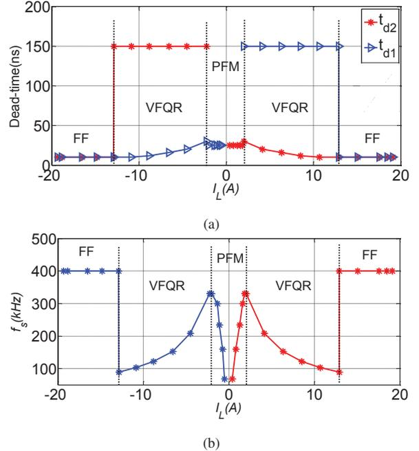
Fig. 9. Measured (a) dead-time and (b) switching frequency in the tri-mode bi-directional converter.
