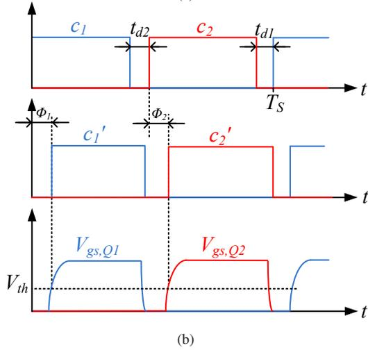
Fig. 4. (a) Simplified architecture of the VFQR controller. (b) Signal timing in VFQR mode.
