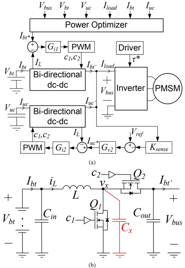
Fig. 1. (a) Architecture of a hybrid energy-storage system. (b) Synchronous boost converter used for interfacing the storage devices to  $V_{bus}$ .
