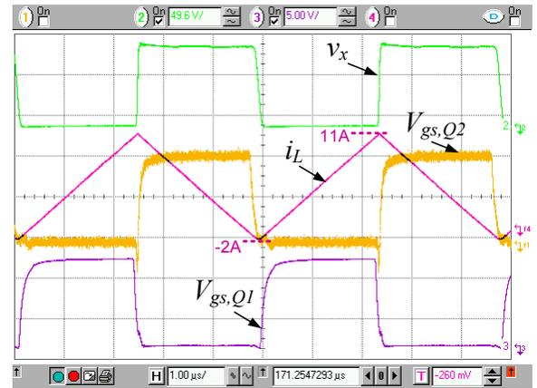
Fig. 6. Measured steady state waveforms of the converter operating in VFQR mode. f-1:  $V_{gs,Q2}$ , 5 V/div; ch-2:  $v_x$ , 49.6 V/div; ch-3:  $V_{gs,Q1}$ , 5 V/div; f-4:  $i_L$ , 5 A/div.
