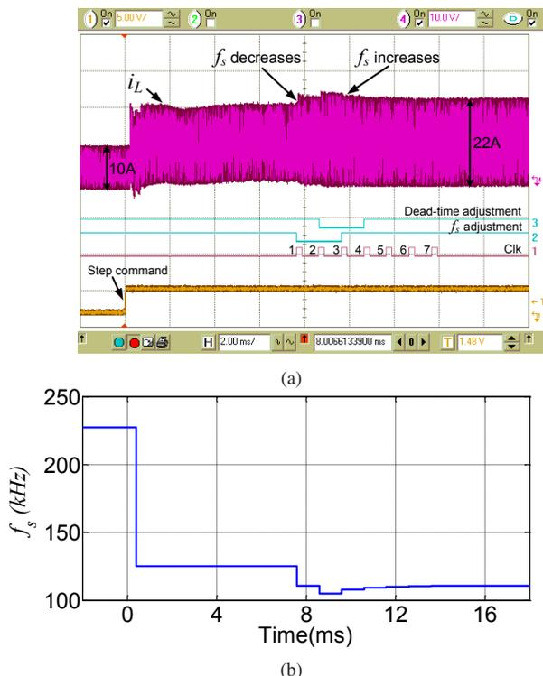
Fig. 11. Measured transient response of the converter due to a step in  $I_{bt}^*$  from 3 A to 9 A. (a) Inductor current and internal digital adjustment signals. ch-4:  $i_L$ , 10 A/div.  $f_s$  adjustment = 0 indicates that the frequency is decreasing. Dead-time adjustment = 0 indicates that the dead-time is increasing. (b) Switching frequency during calibration process.
