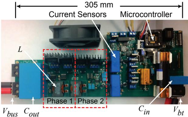
Fig. 5. Fabricated 2 kW quasi-resonant tri-mode converter prototype.
