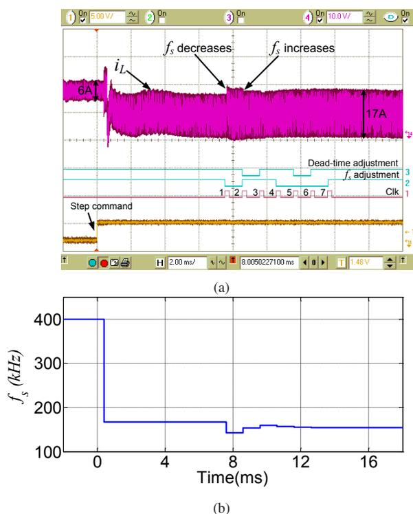
Fig. 10. Measured transient response of the converter due to a step in  $I_{bt}^*$  from 15 A to 6.5 A. (a) Inductor current and internal digital adjustment signals. ch-4:  $i_L$ , 10 A/div.  $f_s$  adjustment = 0 indicates that the frequency is decreasing. Dead-time adjustment = 0 indicates that the dead-time is increasing. (b) Switching frequency during calibration process.
