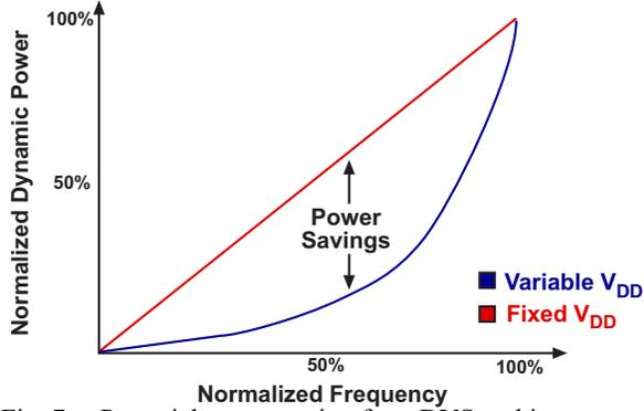
Fig. 7. Potential power saving for a DVS architecture.
