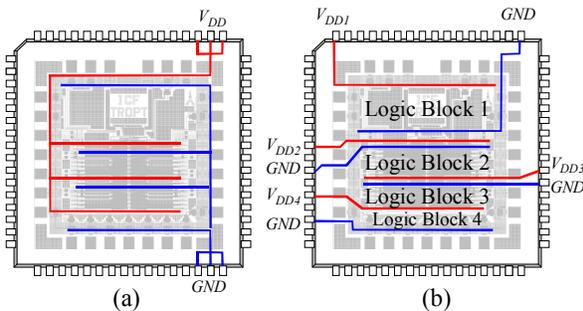
Fig. 4. (a) Conventional power lines inside a VLSI chip. (b) Multiple supply grids powering different circuit blocks inside a VLSI chip.
