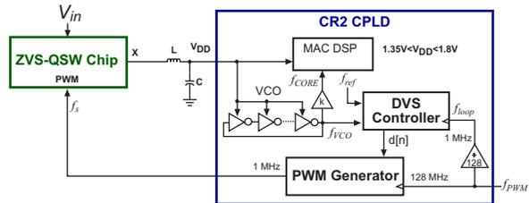
Fig. 11. A dynamic voltage scaling control loop. The unit under test is a Xilinx CoolRunnerII<sup>TM</sup> CPLD configured to represent a typical DSP load using 8 MAC blocks.
