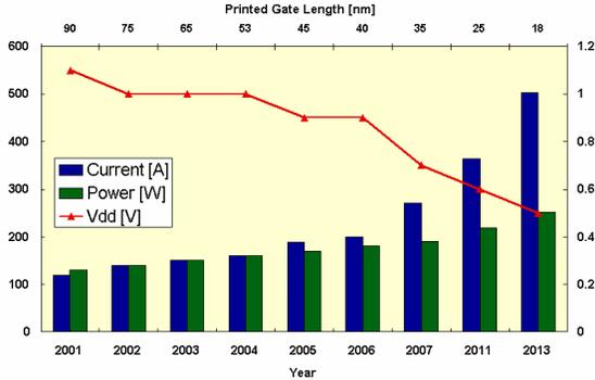
Fig. 3. ITRS Roadmap on supply voltage, current and power requirements.
