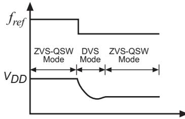
Fig. 13. Representation of a dual mode controller. The DVS loop is only used periodically to update the voltage reference for the ZVS-QSW loop when a new reference frequency is asserted.
