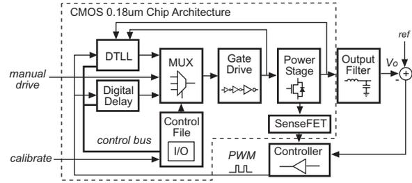
Fig. 9. Block diagram of the ZVS-QSW soft-switching DC-DC converter chip. Circuit blocks outside the dashed-box are off-chip components.
