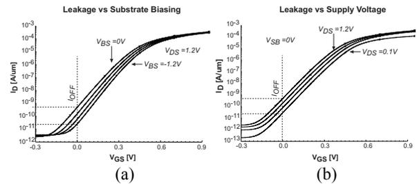
Fig. 2. Simulated drain leakage current in 0.13 $\mu\text{m}$  MOSFETs as functions of (a) substrate bias - hence  $V_{TH}$ , and (b) supply voltages -  $V_{GS}$ .
