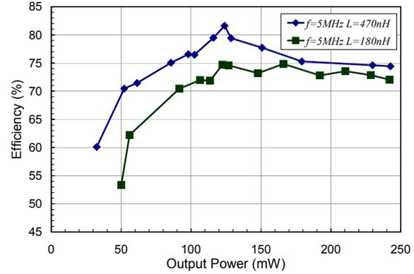
Fig. 10. Measured efficiency of the experimental ZVS-QSW converter for  $V_{in} = 2\text{V}$ ,  $V_o = 1.4\text{V}$ .
