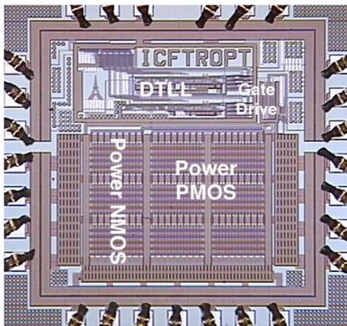
Fig. 8. Micrograph of a ZVS-QSW soft-switching DC-DC converter with precision dead time control. This chip was implemented in 0.18 $\mu\text{m}$  CMOS technology. Die size is 1.25 $\times$ 1.25 mm<sup>2</sup>.
