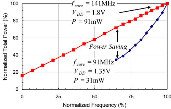
Fig. 12. Measured power savings for the MAC DSP module using the DVS scheme.
