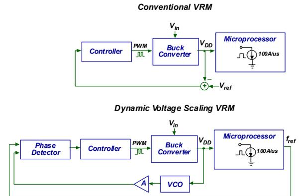
Fig. 6. A comparison between a conventional VRM and Dynamic Voltage Scaling VRM architecture.
