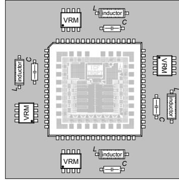
Fig. 5. A VLSI chip module with multiple VRMs to deliver power to the internal circuit blocks.
