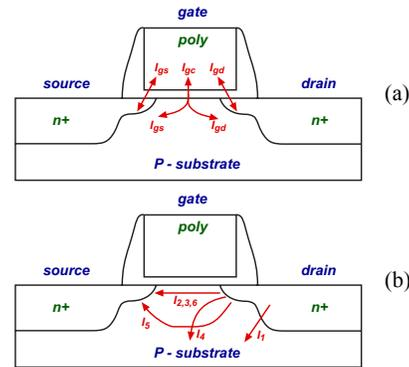
Fig. 1. Gate leakage (a) and off-state drain leakage (b) components in deep sub-micron MOSFETs with ultra-thin oxides.
