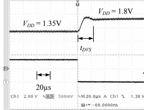
Fig. 14. Measured  $V_{DD}$  waveform with the digital PID controller.  $V_{DD}$  is scaled between 1.8V and 1.35V in  $22\mu s$ . The lower waveform represents the step in  $f_{ref}$ .
