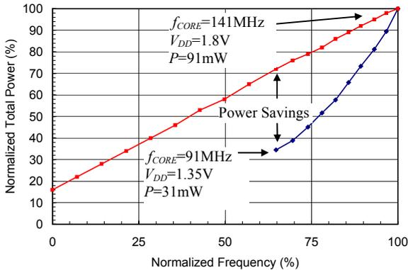
Fig. 16. Measured power savings for the MAC DSP module using the DVS scheme.
