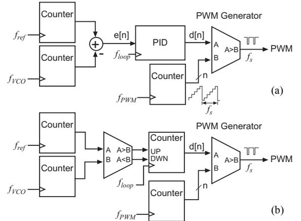
Fig. 7. (a) DVS controller using digital PID and (b) non-linear bang-bang controller.
