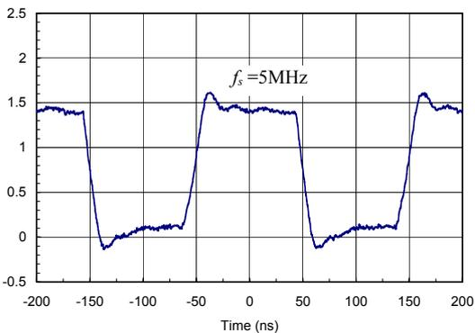
Fig. 14. Measured voltage waveform at node X of the ZVS-QSW converter. Proper gate-drive timing eliminates body-diode conduction after the resonant transitions.
