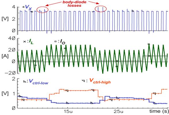
Fig. 5. HSPICE Transient waveforms of ZVS-QSW buck converter with DTLLs under a dynamic load (1.5A-10A).
