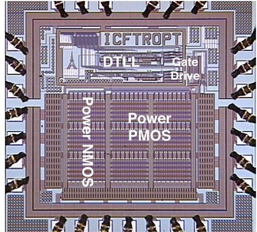
Fig. 10. A micrograph of the 0.18 $\mu\text{m}$  CMOS integrated ZVS-QSW DC/DC converter chip. Die area is 1.56mm<sup>2</sup>.
