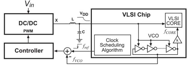
Fig. 8. Simplified block diagram of DVS feedback loop.
