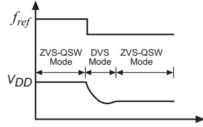
Fig. 9. Representation of a dual mode controller. The DVS loop is only used periodically to update the voltage reference for the ZVS-QSW loop when a new reference frequency is asserted.
