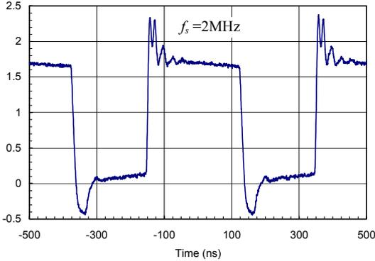
Fig. 13. Measured voltage waveform at node X of the ZVS-QSW converter. Manual gate-drive timing is used to show the body-diode conduction.
