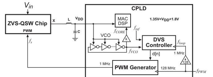
Fig. 15. Implementation of the DVS system using a XC2C256 Xilinx CPLD. The CPLD can function with a core voltage between 1.35V and 1.8V.
