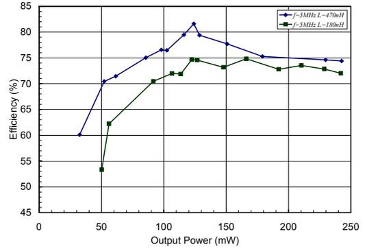
Fig. 12. Measured efficiency of the experimental ZVS-QSW converter for  $V_{in}=2V$ ,  $V_o=1.4V$ .
