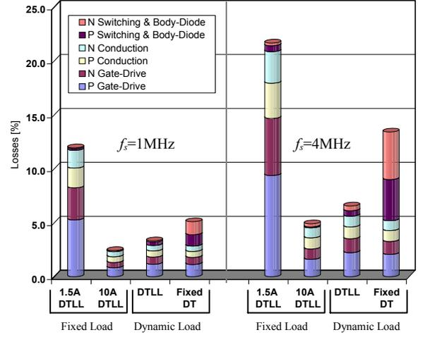
Fig. 6. On-Chip losses with DTLL/ fixed dead-time.  $V_o = 1.3V$ , devices optimized @10A, for 1 and 4MHz.
