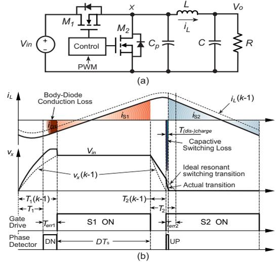
Fig. 2. (a) ZVS-QSW buck converter. (b) Load transient leads to dead-time errors and switching loss. The period  $k-1$  has ideal dead-times.
