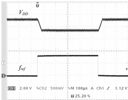
Fig. 17. Measured  $V_{DD}$  waveform with the bang-bang DVS controller.  $V_{DD}$  is scaled between 1.8V and 1.35V in 36 $\mu$ s. The lower waveform represents the step in  $f_{ref}$ .
