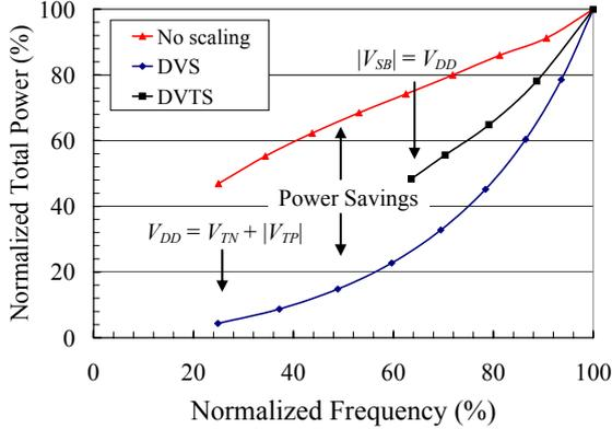
Fig. 1. Normalized simulated power savings for a  $0.18\mu\text{m}$  CMOS ring oscillator using DVS and DVTS.
