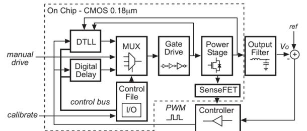
Fig. 11. Block diagram of the ZVS-QSW buck converter chip with integrated DTLLs.
