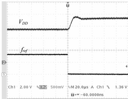
Fig. 18. Measured  $V_{DD}$  waveform with the digital PID controller.  $V_{DD}$  is scaled between 1.8V and 1.35V in 22 $\mu$ s. The lower waveform represents the step in  $f_{ref}$ .
