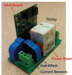
Fig. 3. Assembled Power and DAQ boards.
