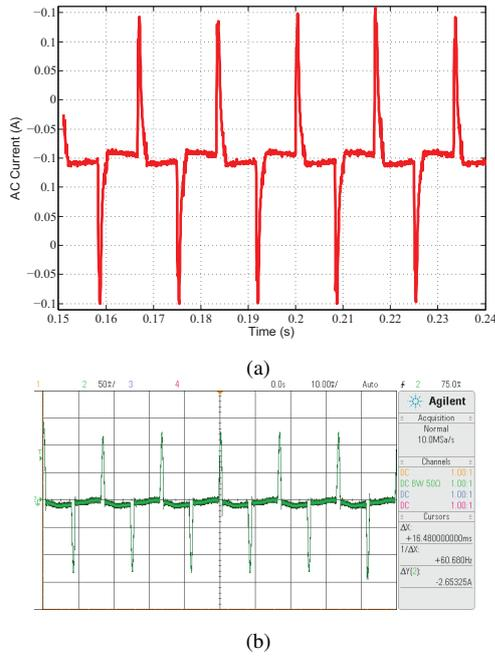
Fig. 8. (a) The AC current measurement, and (b) the reconstructed waveform for a typical 60 W laptop charger in idle state (not charging).
