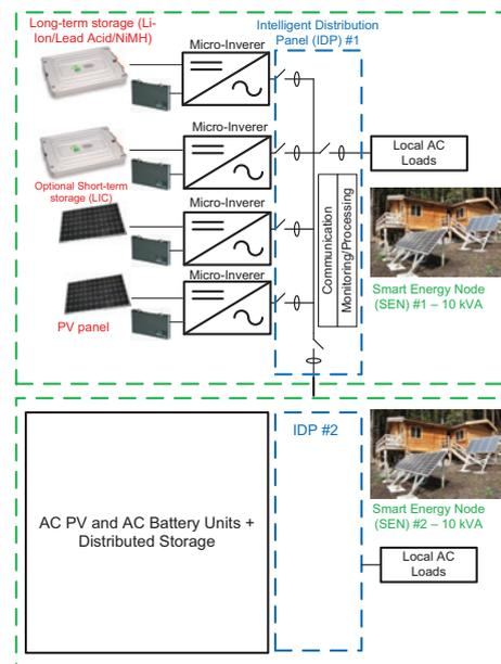
Fig. 1. Proposed nano-grid architecture.
