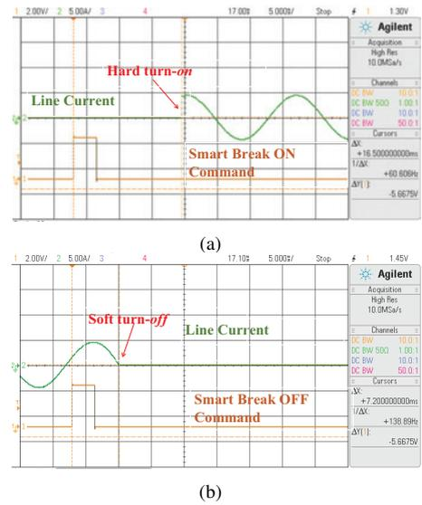
Fig. 9. The smart breaker command and AC line current when (a) connecting, and (b) disconnecting the channel.
