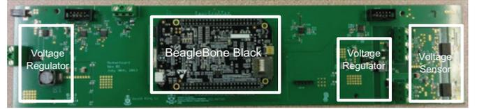
Fig. 4. The IDP motherboard PCB (top view).
