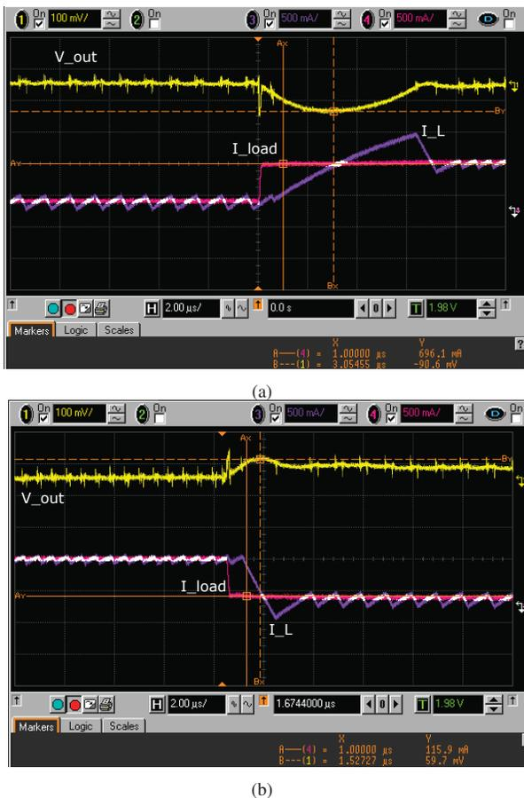
Fig. 8. Dynamic response to (a) a positive load step, and (b) a negative load step using time optimal control. Cursor A shows the step current and cursor B shows the voltage spike or droop.
