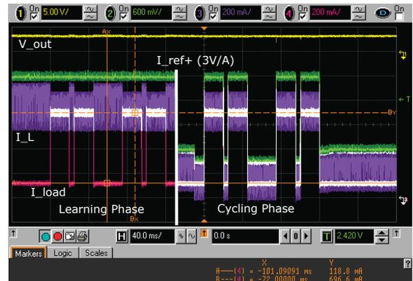
Fig. 10. Learning algorithm in operation: actual load step timings and magnitudes were taken from characterization of the XBee Pro S5 load profile.
