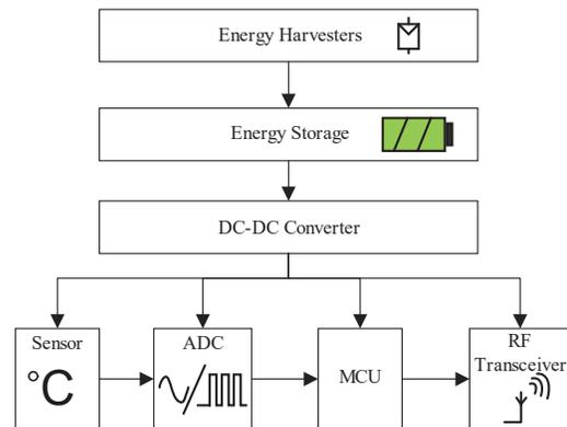
Fig. 1. Simplified IoT-WSN hardware architecture.
