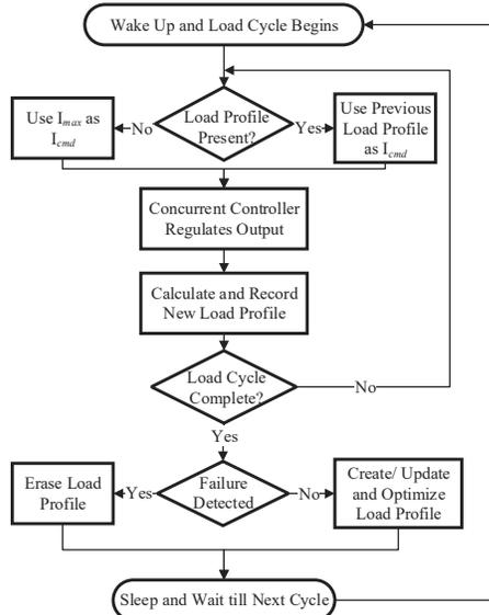
Fig. 6. Preemptive control scheme, including the load forecast calibration process.
