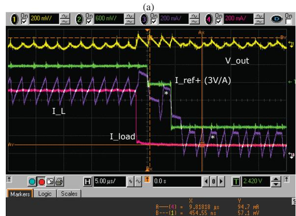
Fig. 9. Dynamic response to (a) a positive load step and (b) a negative load step using preemptive concurrent control. Cursor A shows the step current and cursor B shows the voltage spike or droop, asterisks indicate examples of freewheeling events.
