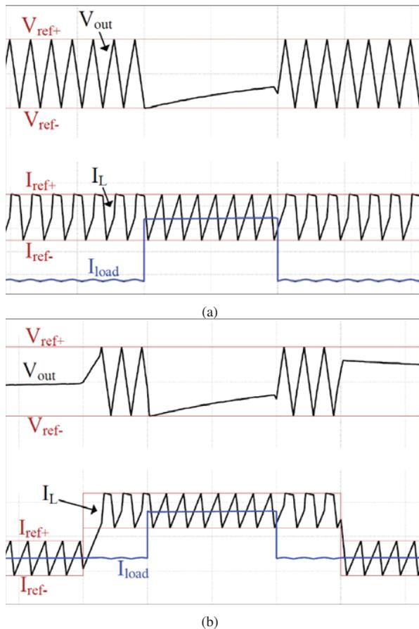
Fig. 5. PCC operation in buck mode (a) prior to calibration, with excessive freewheeling and (b) post-calibration, with adjusted reference current timing such that freewheeling is minimized and efficiency maximized.  $I_{ref+}$ ,  $I_{ref-}$ ,  $V_{ref+}$ , and  $V_{ref-}$  refer to the hysteretic control band limits around  $I_{cmd}$  and  $V_{cmd}$ .
