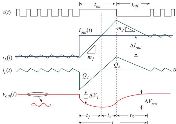
Fig. 3. Conventional time-optimal control waveforms in a buck converter. With this non-linear control, the response time is primarily limited by the inductance value.
