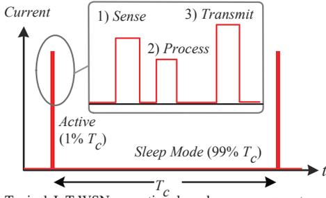
Fig. 2. Typical IoT-WSN operational cycle: measurement, processing and wireless transmission steps.
