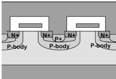
**Fig. 6** Schematic cross-section of a modified *n*-VDMOS with buried  $p^+$ -layer placed underneath the  $n^+$  source
