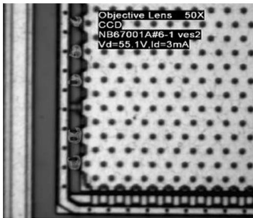
**Fig. 5** Photo-emission analysis of an experimental device with breakdown occurring at the periphery, indicating possible parasitic *npn* turn-on during UIS testing
