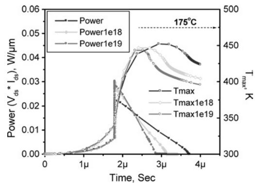
**Fig. 11** Transient of instantaneous power consumption and maximum lattice temperature during UIS switching of devices with different  $p^+$ -strip peak concentrations
