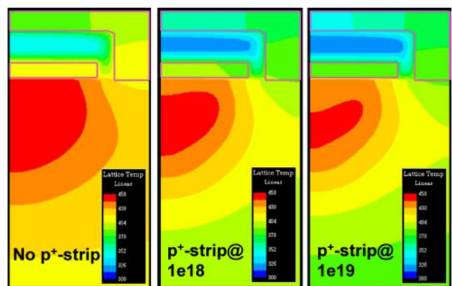
**Fig. 12** Temperature contours of devices with different  $p^+$ -strip peak concentrations when  $T_{max}$  reaches its peak during UIS simulation
