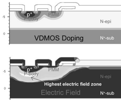
**Fig. 1** Simulated *n*-VDMOS structure and its electric field distribution at a breakdown voltage of 65 V
