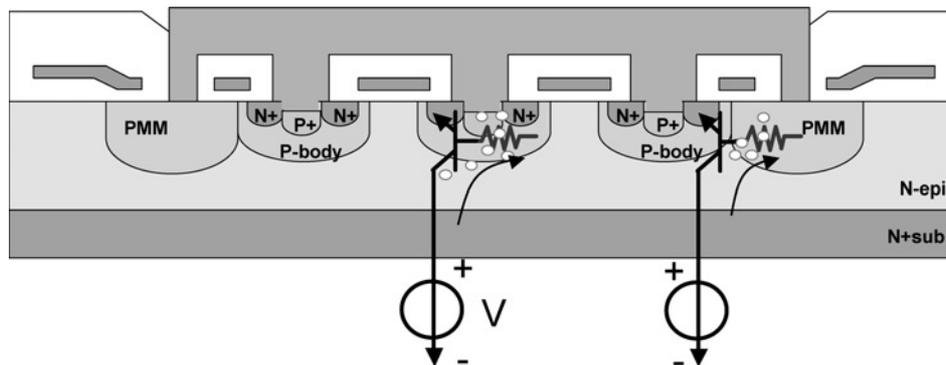
**Fig. 4** Schematic diagram of turning-on parasitic drain-body-source *n**p**n* BJT in a VDMOS upon switching
