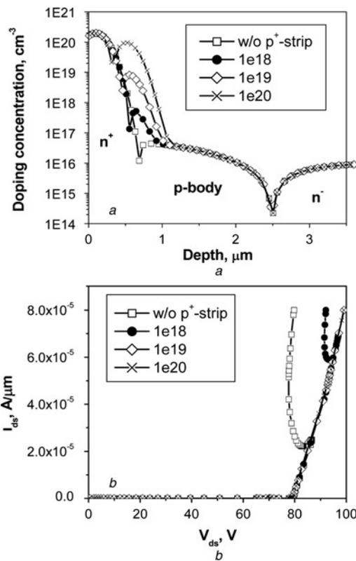
**Fig. 8** Improvement of drain current behaviour by introducing confined  $p^+$ -strip underneath  $n^+$ -source
