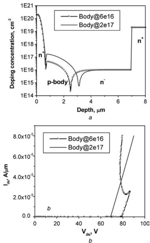
**Fig. 9** Improvement of drain current behaviour by increasing  $p$ -body peak concentration
