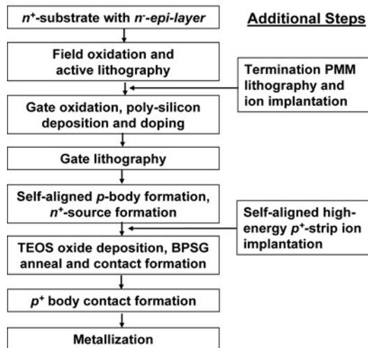
**Fig. 2** AKM VDMOS process flow with additional steps to enhance device ruggedness
