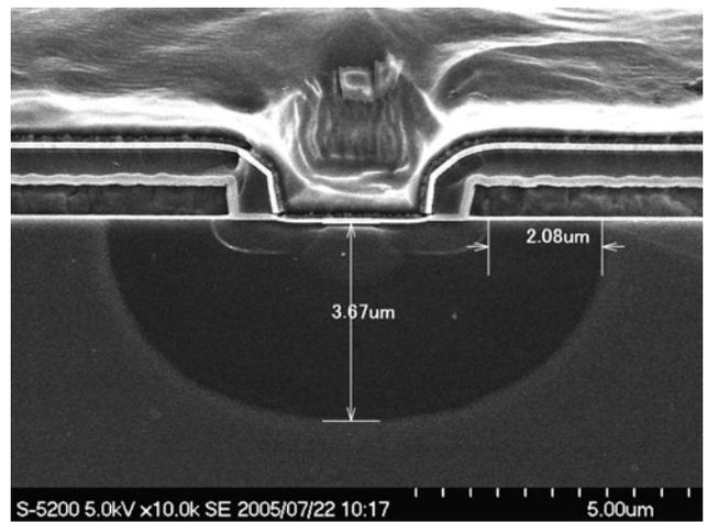
**Fig. 3** SEM cross-sectional structure of a fabricated *n*-VDMOS
