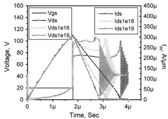
**Fig. 10** Waveform of devices with different  $p^+$ -strip peak concentrations during UIS switching
