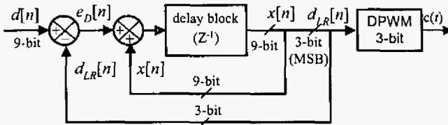
Fig.2. Block diagram of a multi-bit sigma-delta DPWM ( $\Sigma$ - $\Delta$  DPWM).
