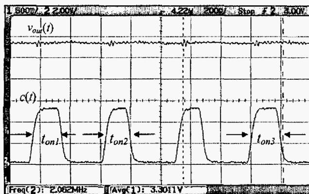
Fig. 6. Steady-state closed-loop operation of the  $\Sigma$ - $\Delta$  DPWM controller at 2.06 MHz switching frequency for  $V_{in}=8$  V. Ch.1: Output voltage  $v_{out}(t)$  (500mV/div); Ch.2: Pulse width modulated control signal  $c(t)$ . Time scale is 200ns/div.
