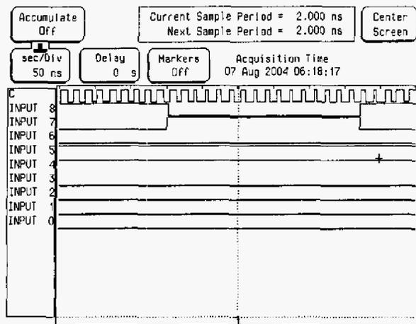
Fig. 5. Pulse width modulated waveforms at 60 MHz produced by  $\Sigma$ - $\Delta$  DPWM (logic analyzer snapshot). *c*- pulse width modulated output signal; inputs 0 to 8 create binary control value  $d[n]$ .
