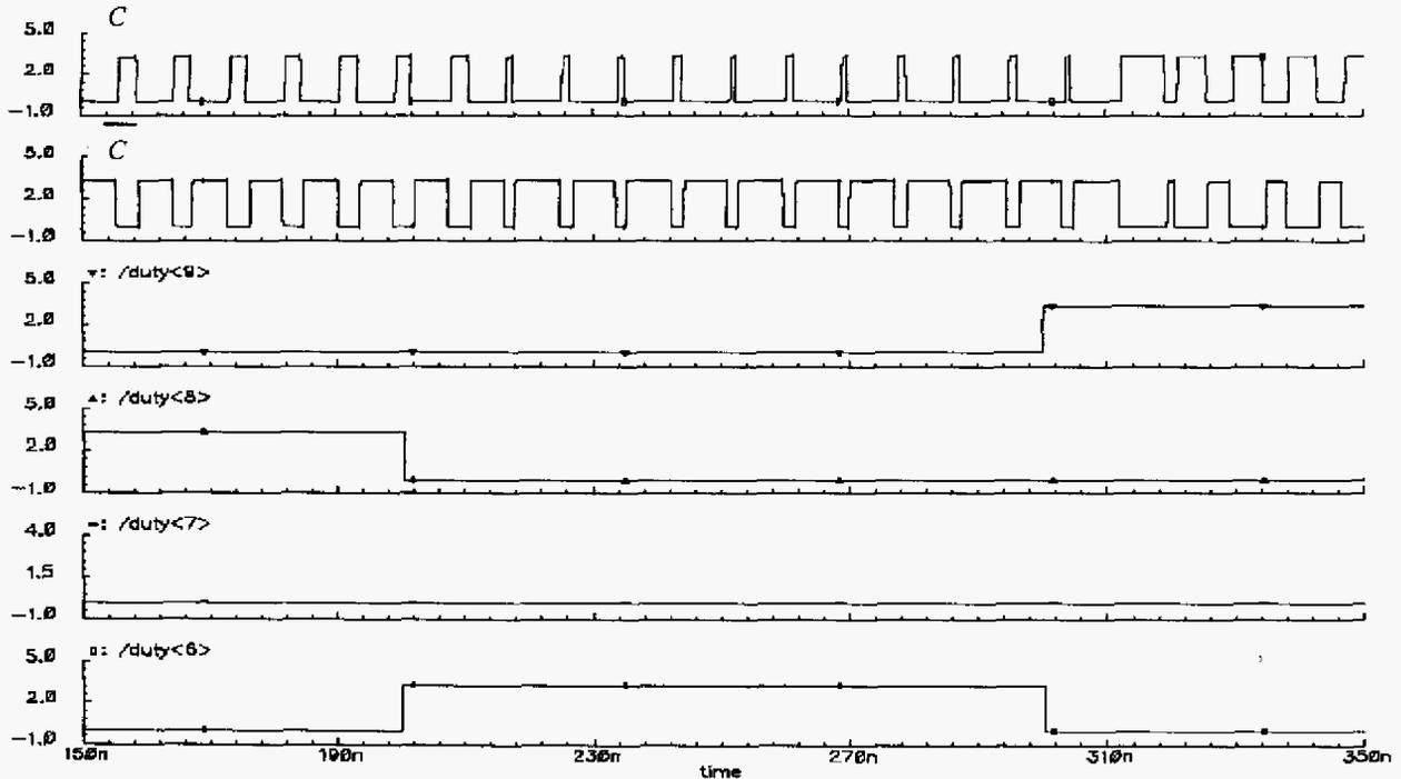
Fig. 9. Simulation results: pulse-width modulated waveforms at 115 MHz produced by the  $\Sigma$ - $\Delta$  DPWM IC.  $C$  and  $\bar{C}$  are the outputs of the dead-time circuit (Fig.4); Duty 6 to 9 are 4 most significant bits of the 10-bit input control value  $d[n]$ .
