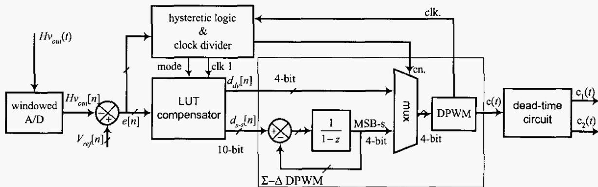
Fig.4. Dual-sampling mode digital compensator.
