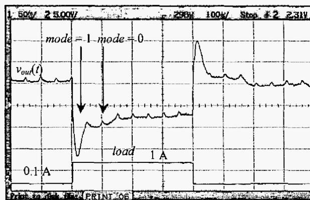
Fig. 7. Transient response for the load change between 0.1 and 1A. Ch.1: Output voltage  $v_{out}(t)$  (50 mV/div – ac scale); Ch.2: load transient. Time scale is 100  $\mu$ s/div.
