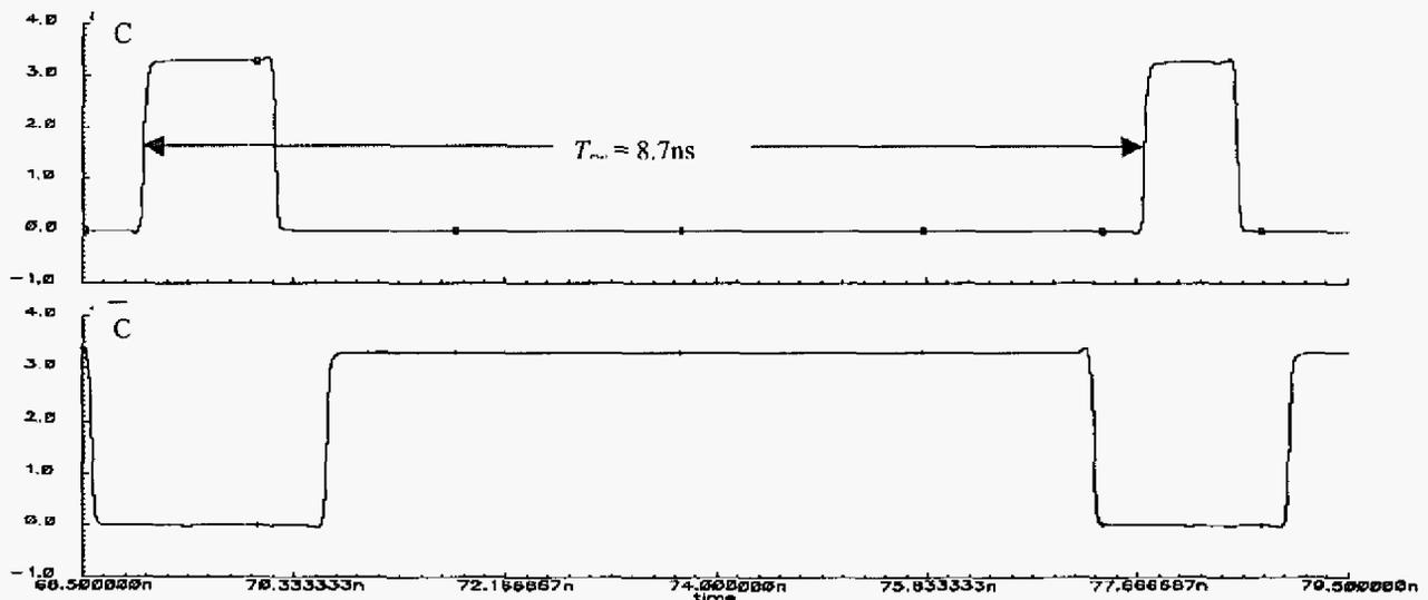
Fig.10. Simulation results: pulse-width modulated waveforms at 115 MHz produced by the  $\Sigma$ - $\Delta$  DPWM IC. C and  $\bar{C}$  are the outputs of the dead-time circuit.  $T_{DPWM}$  is the period of the DPWM.
