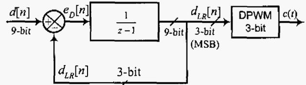
Fig.3. Dynamic model of the  $\Sigma$ - $\Delta$  DPWM.
