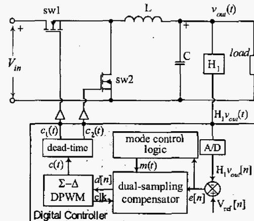
Fig. 1. A buck converter regulated with  $\Sigma$ - $\Delta$  DPWM controller.
