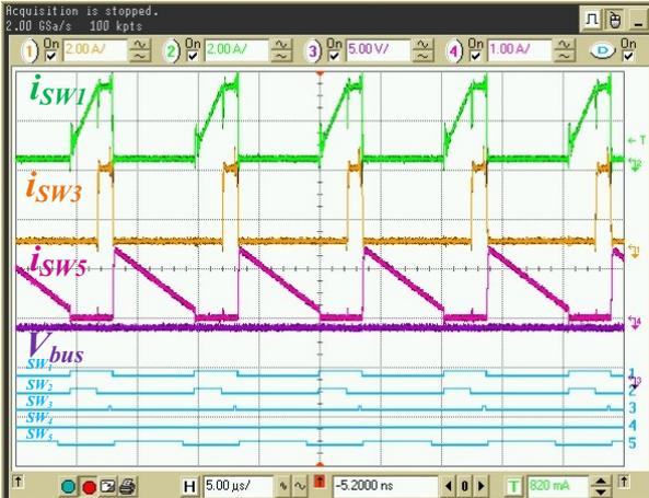
Fig.8: Steady-state operation in battery charging mode, when  $V_{adap}=9V, V_{batt}=7.5V, V_{bus}=5V$
