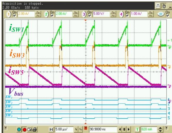
Fig.6: Steady-state operation in battery charging mode, when  $V_{adap}=9V, V_{batt}=3V, V_{bus}=5V$
