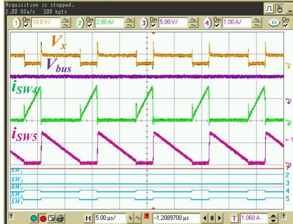
Fig.10: Steady-state operation from battery input, when  $V_{batt}=7.5V, V_{bus}=5V$
