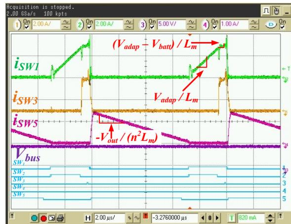
Fig.7: Magnified steady-state operation in battery charging mode, when  $V_{adap}=9V, V_{batt}=3V, V_{bus}=5V$
