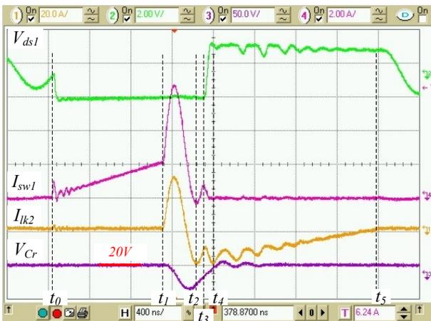
Fig.9. Steady-state operation of soft-switched flyback converter.  $i_{lk2}$  is the transformer secondary side current,  $v_{ds1}$  is the voltage across flyback converter main switch,  $SW_1$ , and  $v_{Cr}$  is the voltage across the resonant circuit capacitor.
