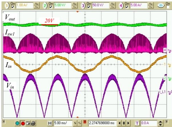
Fig.8. PFC operation of the soft-switched flyback converter.
